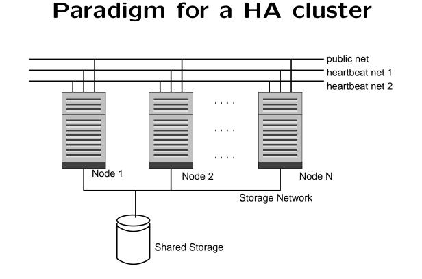
Consists of multiple local machines, LAN networked with some type of shared storage (either parallel SCSI, Fibre Channel or NAS).
